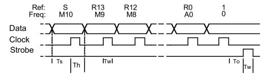
Set-up time (Ts), Hold time (Th), Clock and Strobe pulsewidths (Tw) and Strobe offset time (To) all to be greater than 100 nanosec.
