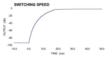
Measured using HP8561E Spectrum Analyser RBW 1 kHz, VBW 1 kHz, Span 0 Hz, Swp 50 ms.
